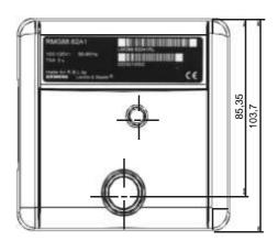
Burner control complete with lockout reset button extension AGK20.43 and plug-in base
