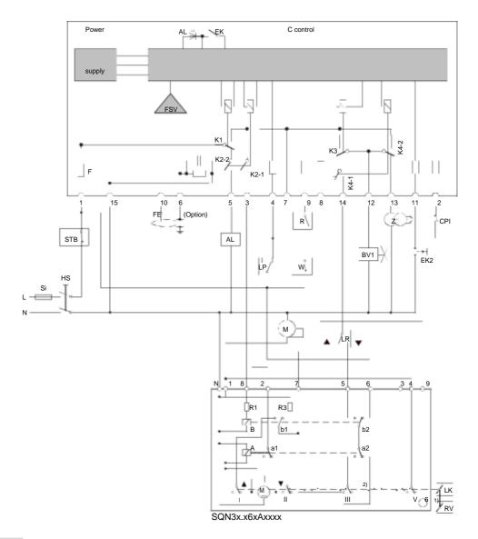
If the contacts of switch V welded in position 49, supervision of the ignition load position would be negated and would not be detected in operation. This means that the circuit welding only used for supervision purposes. The user must ensure that, in the event of failure (should the burner ignite at nominal load «NL»), no damage will occur.
